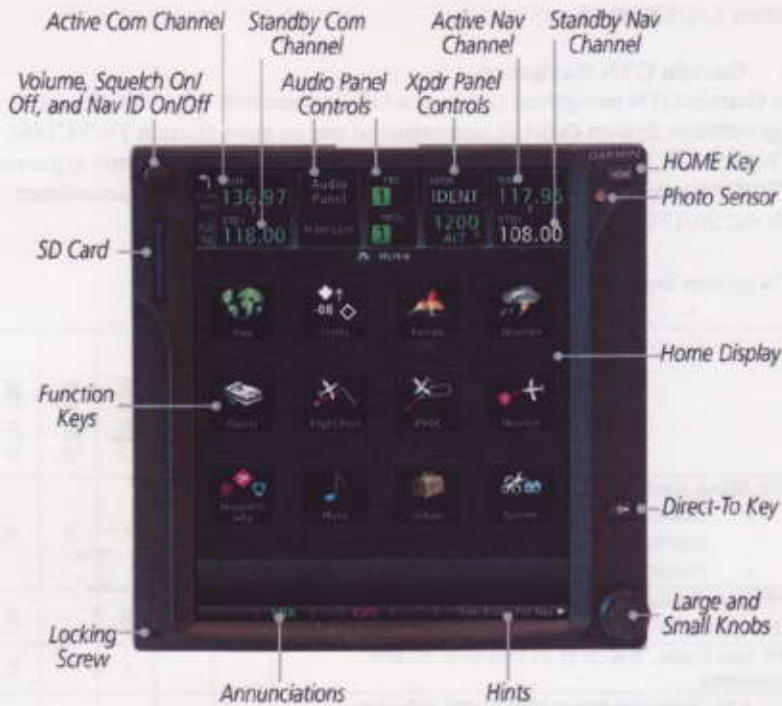
Figure 1 - GTN 750 Control and Display Layout
